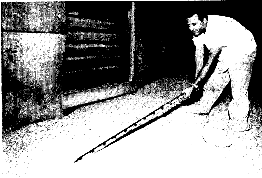
SAMPLER EMPTYING GRAIN SAMPLE FROM PROBE
