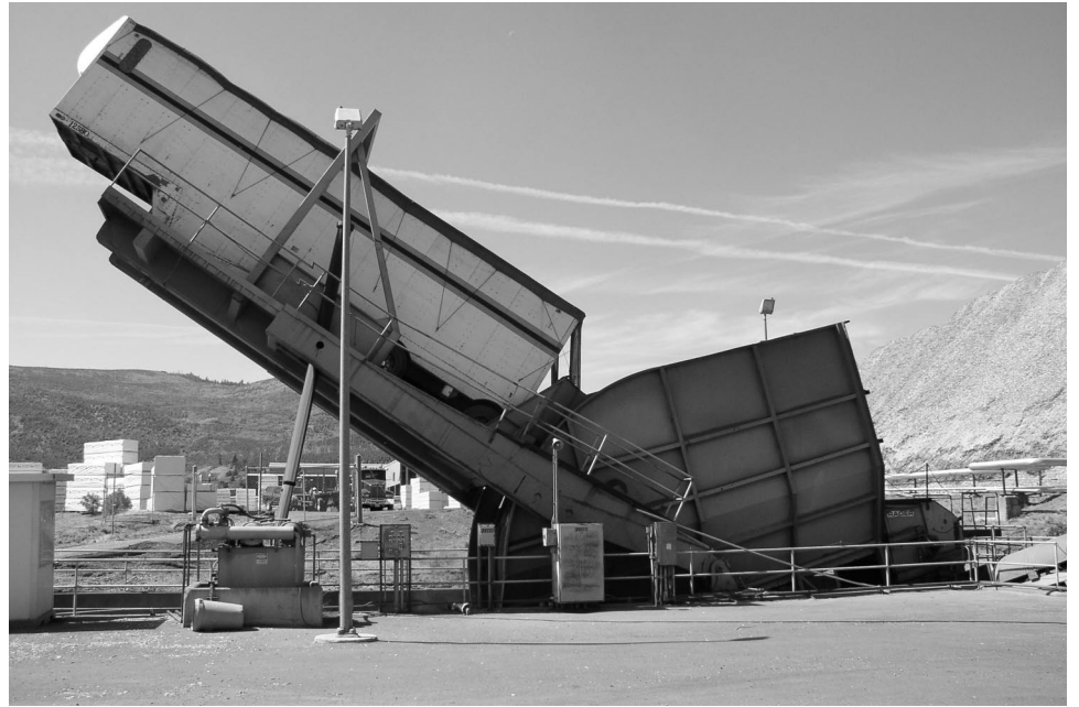
Figure 2: Chip Truck Being Emptied, California Power Plant
