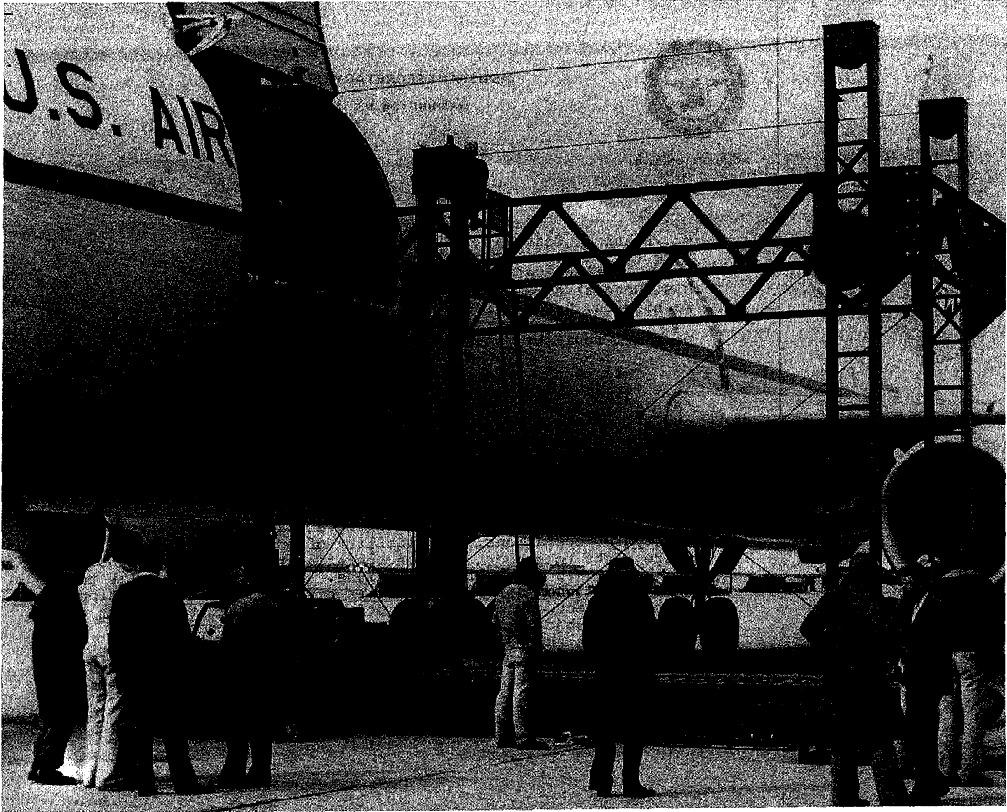
Figure I.4: Wilson Elevator Loader
