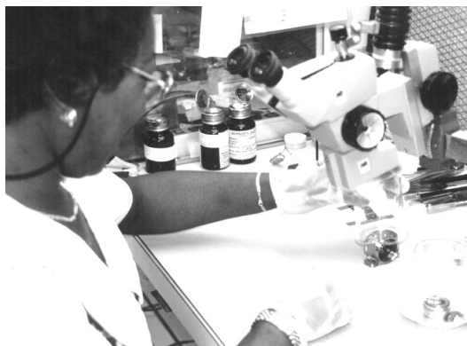
Diagnostic and functional testing on Pendulous Integrating Gyro Accelerometer (PIGA), a component of the minute man inertial guidance system.
