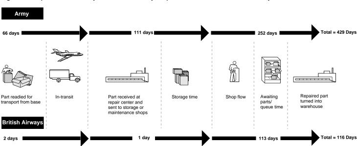
Figure 1: Comparison of the Army's and British Airways' Pipeline Times for a Gearbox Assembly
