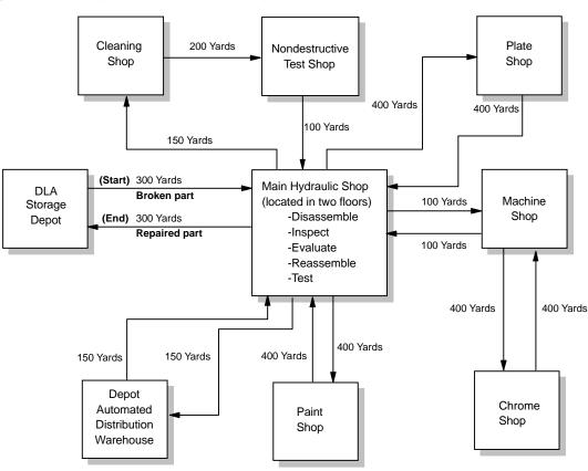
Figure 3: The Army's Repair Process for a Hydraulic Component
