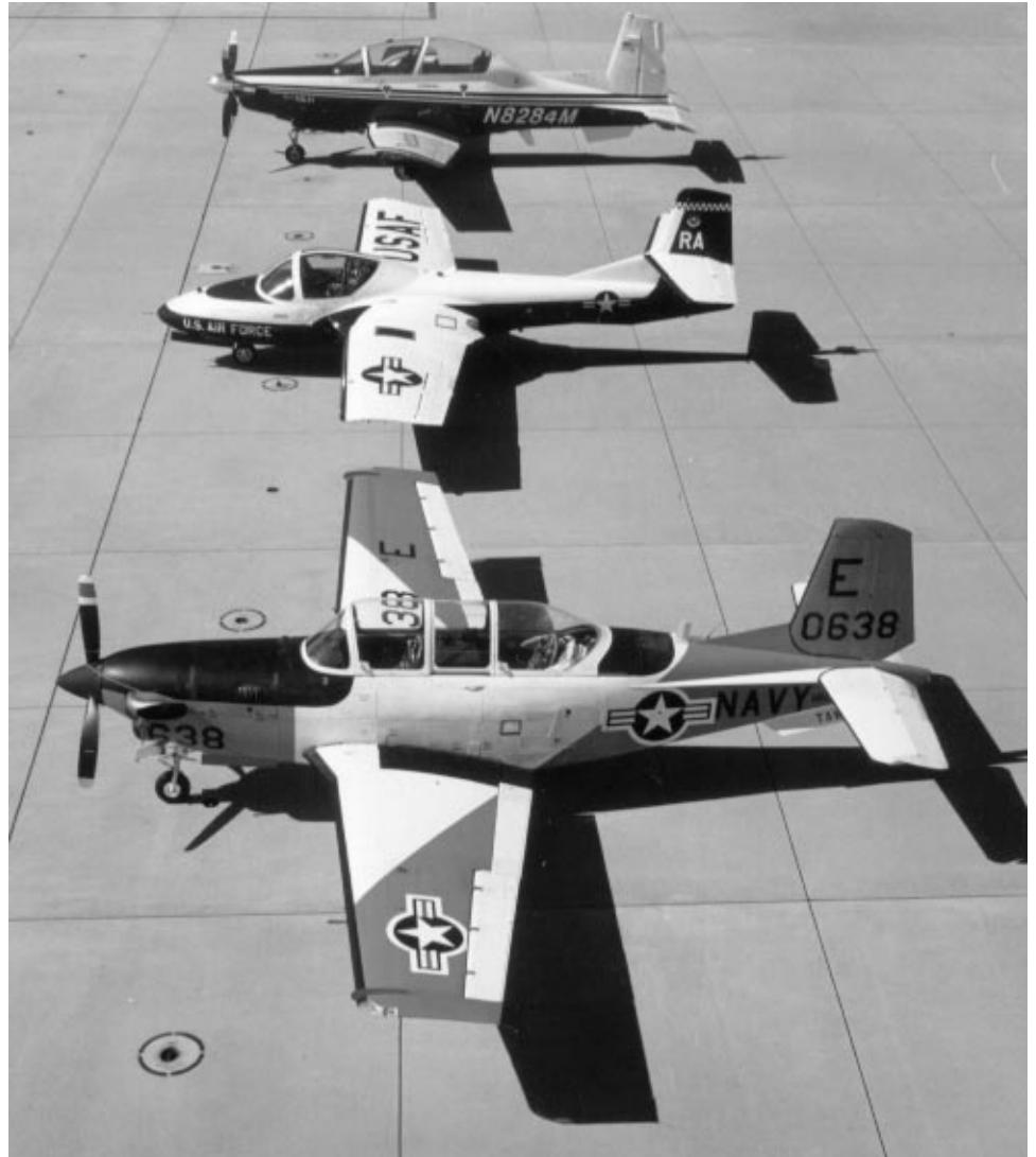
Figure 2: T-6A “Texan II” JPATS, Air Force T-37B “Tweet,” and Navy T-34C “Turbo-Mentor” Training Aircraft (pictured from top to bottom)
