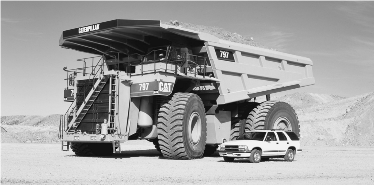
Caterpillar developed the 797, a 360-ton capacity mining truck, in 18 months. Source: Caterpillar, Inc.
