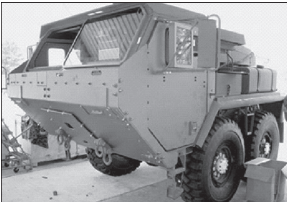
Figure 6: Armored Cab of the Marine Corps Logistics Vehicle System
