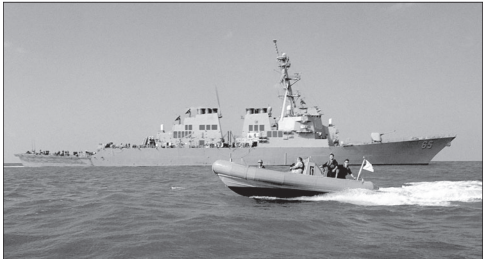
Figure 6: The U.S.S. Benfold , an Arleigh Burke -class Guided Missile Destroyer, with a Rigid Hull Inflatable Boat Passing in the Foreground
