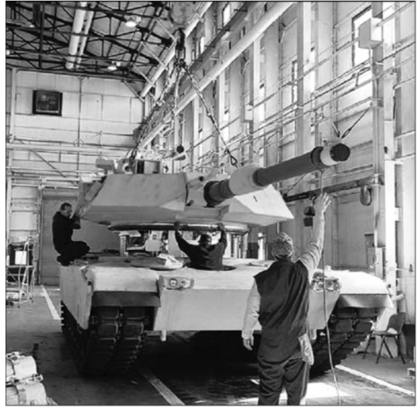
Figure 1: Mechanics at Anniston Army Depot Line Up a Turret with Its Hull
