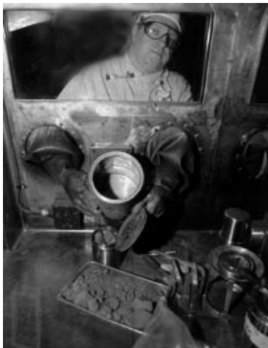
Figure 2.1: A Rocky Flats Worker Handling Plutonium Residues in a Glovebox
