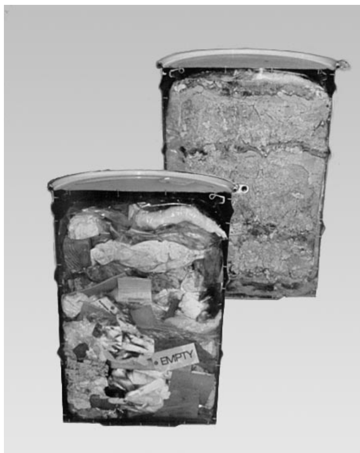
Figure 1.2: Cutaway View of Transuranic Waste Drums
