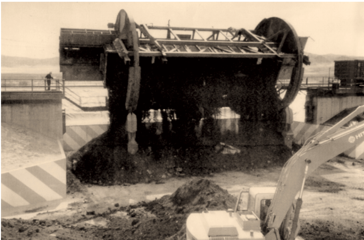
Figure II.5: Unloading Bulk Waste Materials From a Rail Car at the Envirocare Disposal Facility
