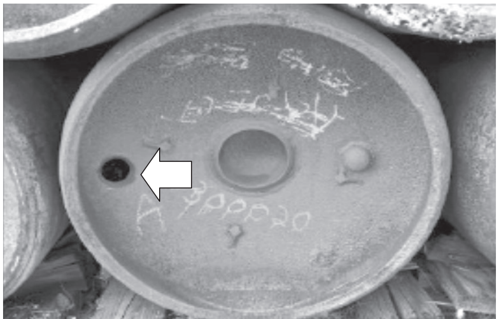
Figure 2: Cylinder with an Open Hole
