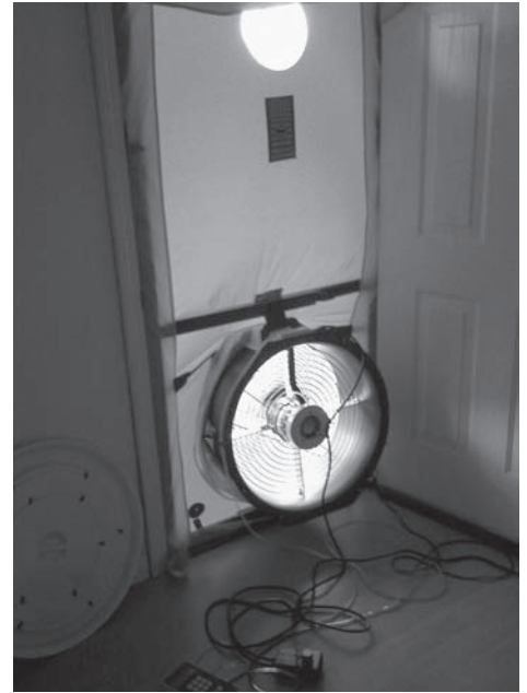
Inside view of blower door set-up
