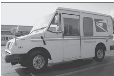
Source: GAO. FFVs have an extra window behind the door for improved visibility.
