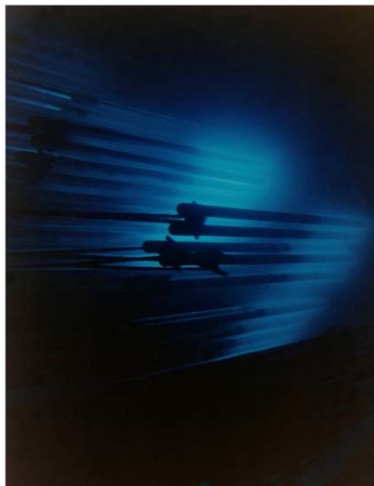
Figure 4.1 Cherenkov radiation illuminating reactor fuel assemblies immersed in water. Source: Photo courtesy of U.S. Department of Energy.
