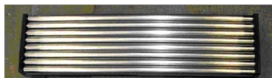
Figure 2.2 Tubes used in a proportional detector for large-area detectors. Source: Oak Ridge National Laboratory.
