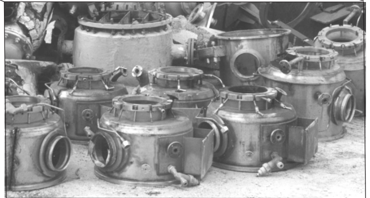
Discarded "Butterfly" Airflow Valves Removed from Building 231.
