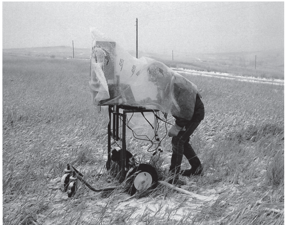
Figure 17: A High-Purity Germanium Detector Can Detect Certain Radionuclides
