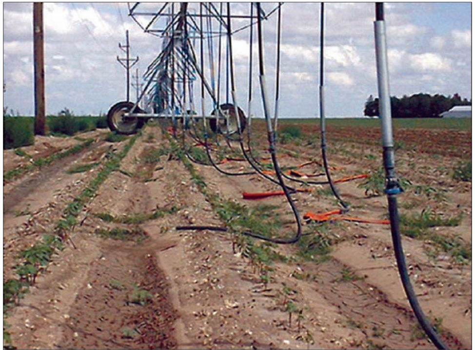
Figure 7: Example of Low-Energy Precision-Application Irrigation
