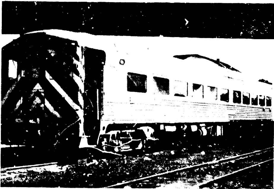
CONRAIL SELF-PROPELLED RAIL CAR USED IN COMMUTER SERVICE
