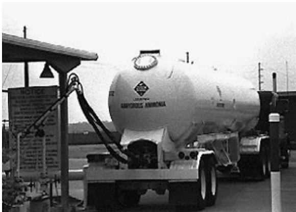
Trucks with pressurized tanks pick up the anhydrous ammonia at the terminal for delivery to dealerships that sell fertilizer to farmers.
