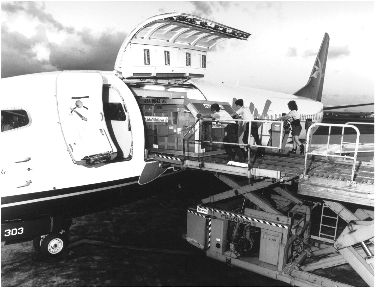
Figure 4: Aloha Airlines Carries Cargo Using Boeing 737s Converted From Passenger Service to Cargo Service
