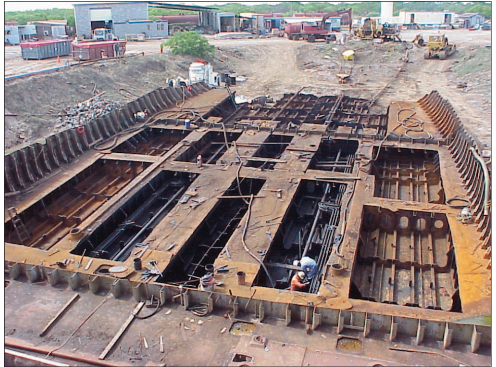
Figure 3: Ship Near End of the Scrapping Process
