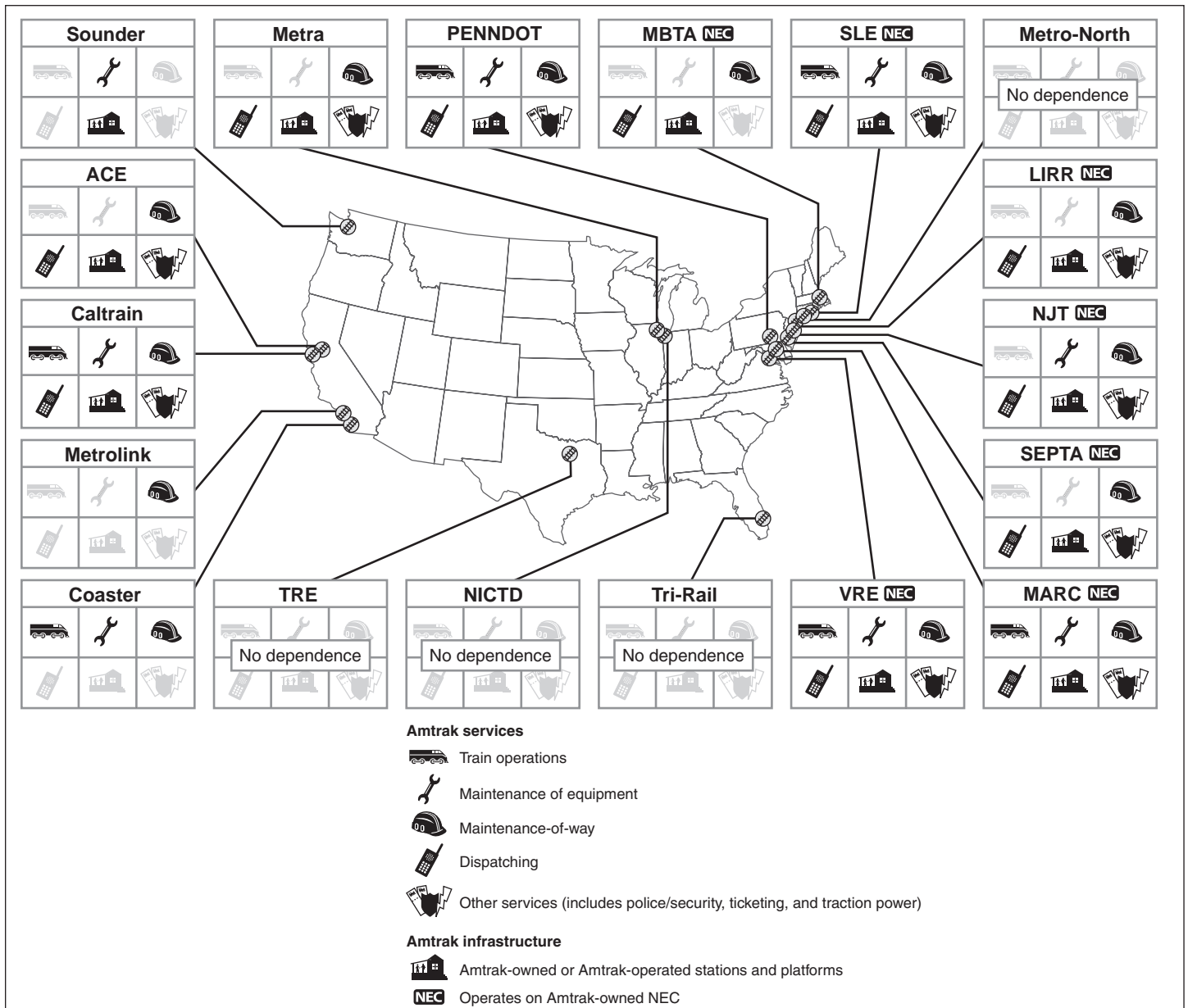
Figure 2: Overview of Commuter Rail Agency Reliance on Amtrak for Infrastructure and Services
