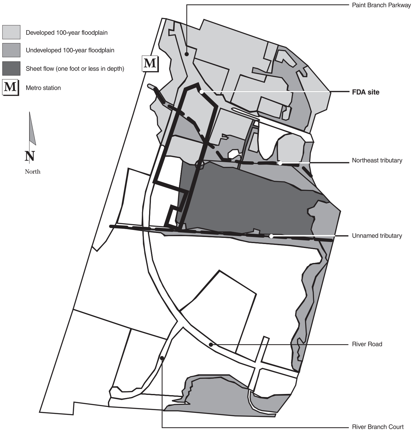
Figure 1: Existing Prince George's County-defined 100-Year Floodplain in Area Surrounding the Proposed FDA Facility
