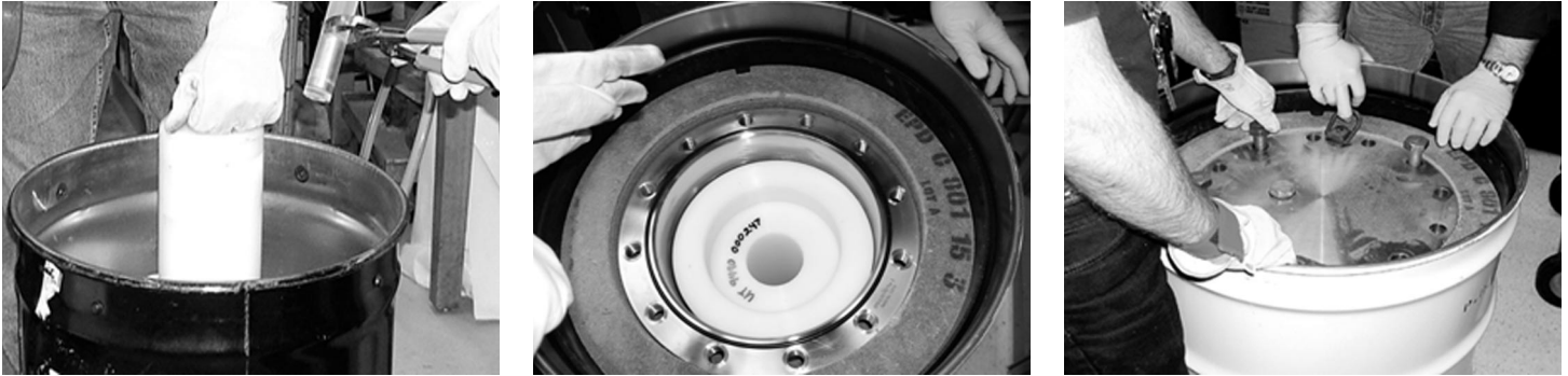
Figure 2: Source Recovery Project Personnel Remove a Sealed Radiological Source and Repackage It into a WIPP-Acceptable Disposal Drum
