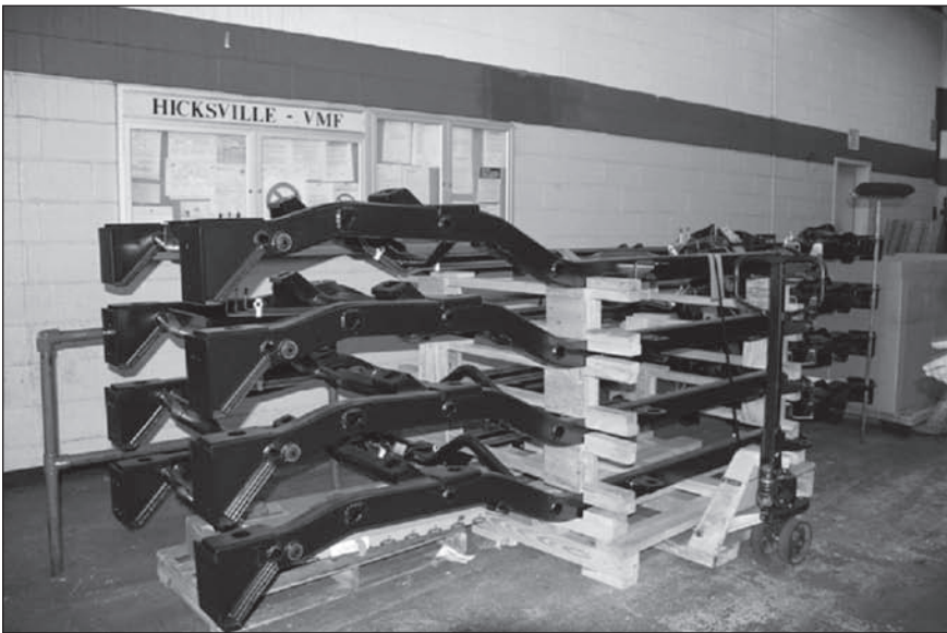
Figure 9: New LLV Frames Awaiting Installation (left), and an LLV Being Reassembled after a Frame Replacement (right), 2010
